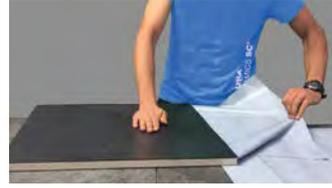
**3** Proceed smoothly until joining adhesion on the entire surface, avoiding wrinkles or air bubbles.
